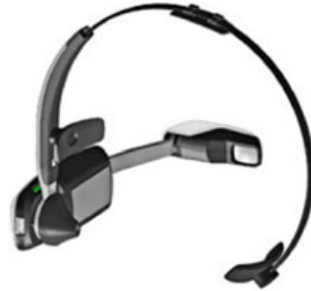
Fig. 3 Vuzix m100 AR headset. The M100 has an onboard 1.2 GHz processor with 1 GB of RAM running Android as its operating system. Its display covers one eye, and has a visibility equivalent to a 4 in. mobile screen held 14 in. away. There is onboard audio for one ear
