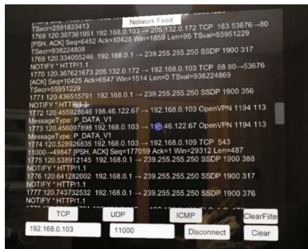
Fig. 8. Network monitoring window running on HoloLens
